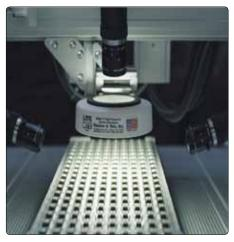
The pressure sensor is 100% inspected for position - missing parts - orientation - glue coverage and more.
