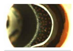
Glue coverage measured in an area tailored to the inspected object
