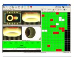
Clicking in the matrix on the screen moves the robot in position and reinspects sensor.
